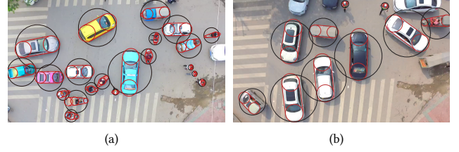
Figure 2: Comparison between the representation of disk (black) and our medial-axis-based representation (CTMAT in red). Our representation is less conservative and can accurately model such dense traffic scenarios. On the other hand, disk-based representations are overly conservative and unable to compute collision free trajectories.
